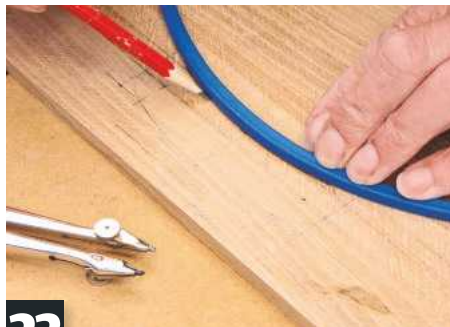
23 Draw handle cutout with flexible curve or arched steel rule. Allow enough width for sanding drum
